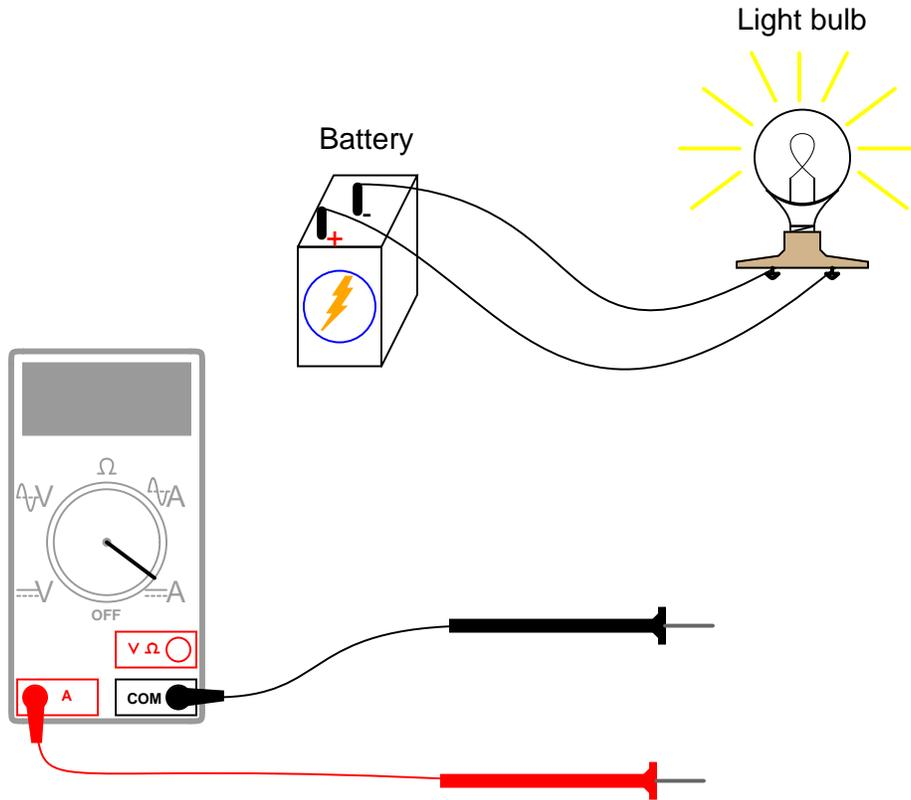
Also, draw a schematic diagram of this same circuit (with the ammeter connected).
