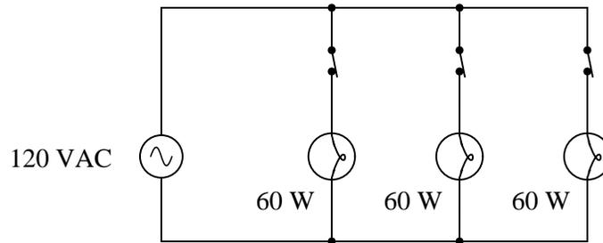
The student uses Joule's Law to calculate the resistance of each lamp ( $240 \Omega$ ), and uses the parallel resistance formula to calculate the circuit's total resistance ( $80 \Omega$ ). With the latter figure, the student also calculates the circuit's total (source) current: 1.5 A.
