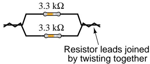
How much electrical resistance would you expect an ohmmeter to indicate if it were connected across the combination of these two parallel-connected resistors?
