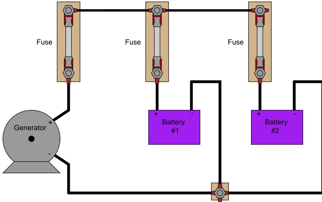
To do so, of course, you need to determine the direction of current through each battery. Unfortunately, your multimeter does not have the current rating necessary to directly measure such large currents, and you do not have access to a clamp-on (magnetic) ammeter capable of measuring DC current.
