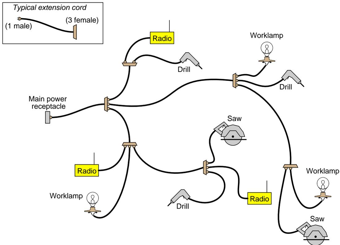
Despite this dangerous wiring, all tools have functioned so far without trouble. Then suddenly both the worklight and the circular saw in the lower-right corner of the illustration stop working. All the other tools continue to function properly (including all the radios, which is very fortunate because the workers become irritable without their music).
