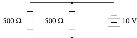
Now, using Ohm's Law, calculate total resistance ( $R_{total}$ ) from total (source) voltage  $V_{total}$  and total (source) current  $I_{total}$ .
