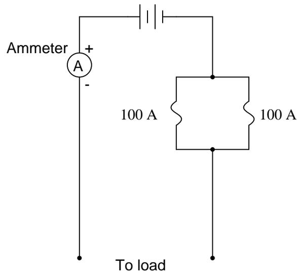
However, after a few years of operation, the system begins blowing fuses even when the ammeter registers less than 200 amps of load current. Upon investigation, it is found that one of the fuse holders had developed corrosion on a terminal lug where one of the wires connects:
