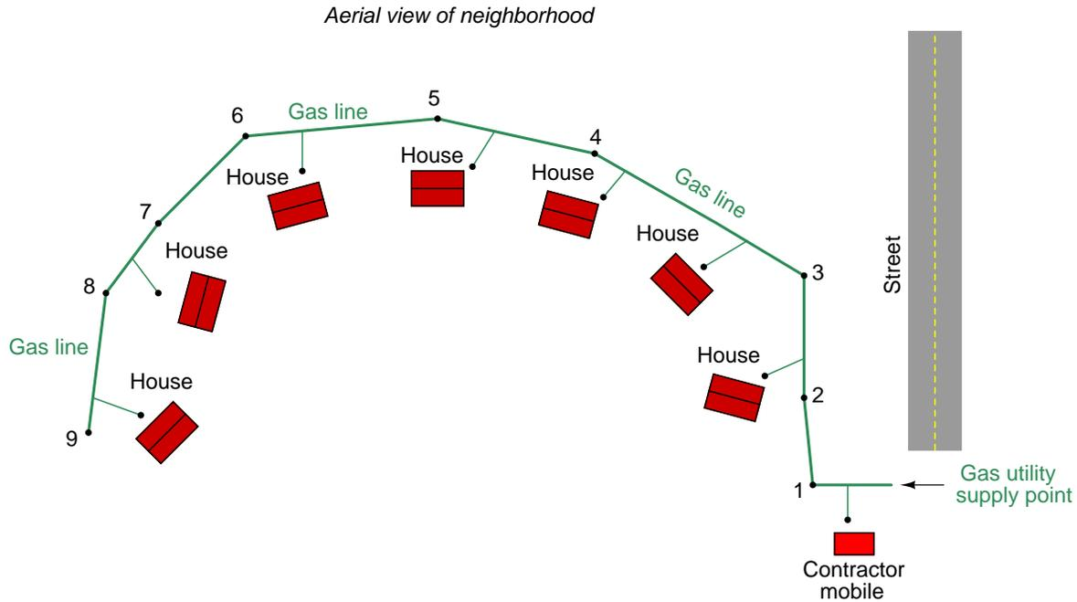
Each black dot on the diagram is a shutoff valve, used for isolating different sections of the service pipeline. Based on the heating technician's report, you conclude that the service pipeline going up to that house must not be "live," and that one of the numbered valves was probably left in the *off* position. But which one could it be?
