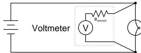
Explain why it is usually safe to ignore the internal resistance of an voltmeter, though, when it is in a circuit. A common term used in electrical engineering to describe this intentional oversight is *swamping*. In this particular circuit an engineer would say, “The resistance of the light bulb *swamps* the internal resistance of the voltmeter.”
