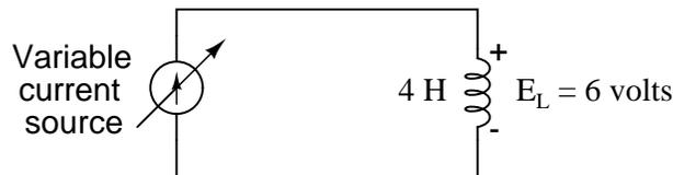
In real life, through, the inductor would drop more than 6 volts, due to winding resistance.
