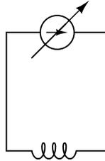
Now, suppose the adjustable current source is steadily *decreased* over time. We know this will result in a magnetic field of decreasing strength in the inductor. Does this decrease in magnetic field constitute an *accumulation* of energy in the inductor, or a *release* of energy from the inductor? In this scenario, does the inductor act as a *load* or as a *source* of electrical energy?
