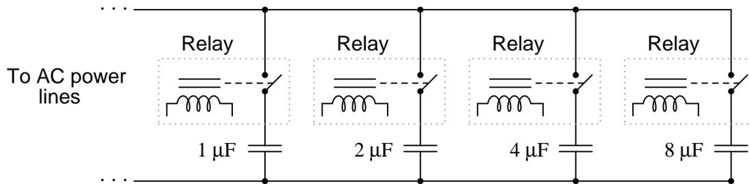
Explain how a circuit such as this provides a step-variable capacitance, and determine the range of capacitance it can provide.
