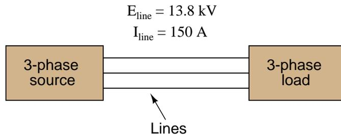
A 13.8 kV single-phase system could be designed to provide the same amount of power to a load, but it would require heavier-gauge (more expensive!) conductors. Determine the extra percentage of expense in wire cost (based on the weight of the wires) resulting from the use of single-phase instead of three-phase.
