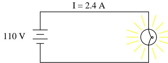
Calculate the power dissipation in this circuit, and describe the transfer of energy from source to load: where does the energy come from and where does it go to?
