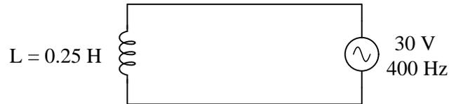
Calculate the apparent, true, and reactive power for this circuit:
