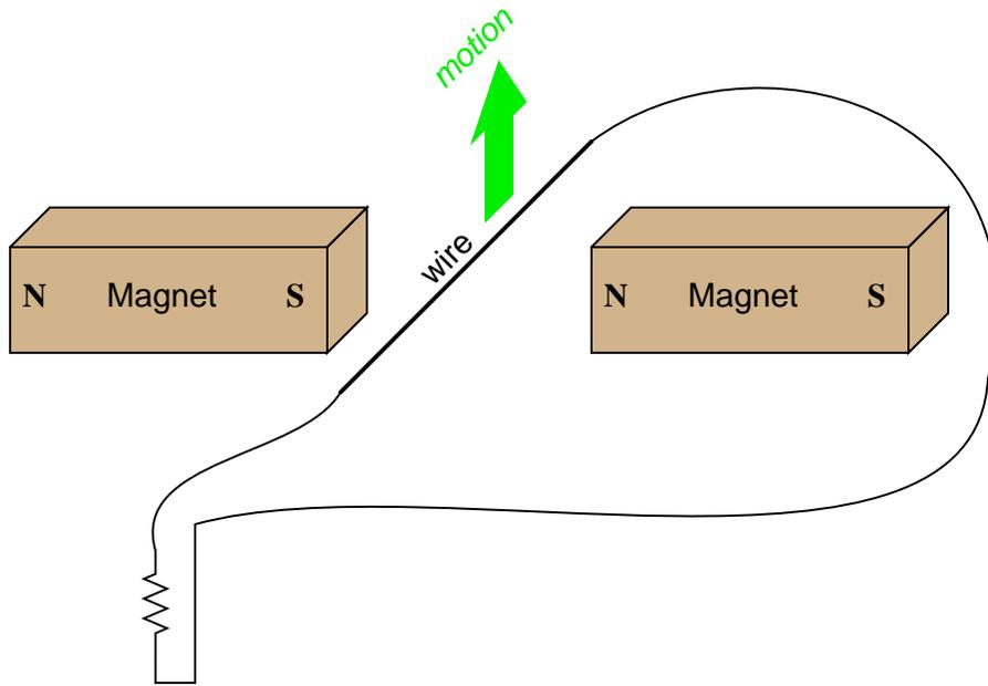
We know that current moving through a wire will create a magnetic field, and that this magnetic field will produce a reaction force against the static magnetic fields coming from the two permanent magnets. Which direction will this reaction force push the current-carrying wire? How does the direction of this force relate to the direction of the wire's motion? Does this phenomenon relate to any principle of electromagnetism you've learned so far?
