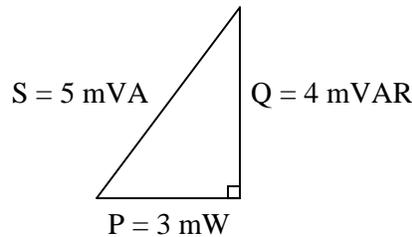
Follow-up question: when making the leap from DC circuit analysis to AC circuit analysis, we needed to expand on our understanding of "opposition" from just resistance ( $R$ ) to include reactance ( $X$ ) and (ultimately) impedance ( $Z$ ). Comment on how this expansion of terms and quantities is similar when dealing with "power" in an AC circuit.
