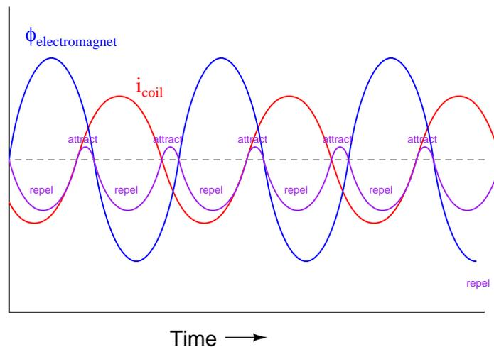
Given a phase shift between the two currents greater than 90 degrees (approaching 180 degrees), there is greater repulsion force for greater duration than there is attractive force. If the coil were a superconducting
