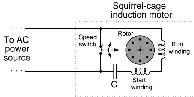
Explain why this special winding is necessary for the motor to start, and also why there is a capacitor connected in series with this start winding. What would happen if the start switch, capacitor, or start winding were to fail open?
