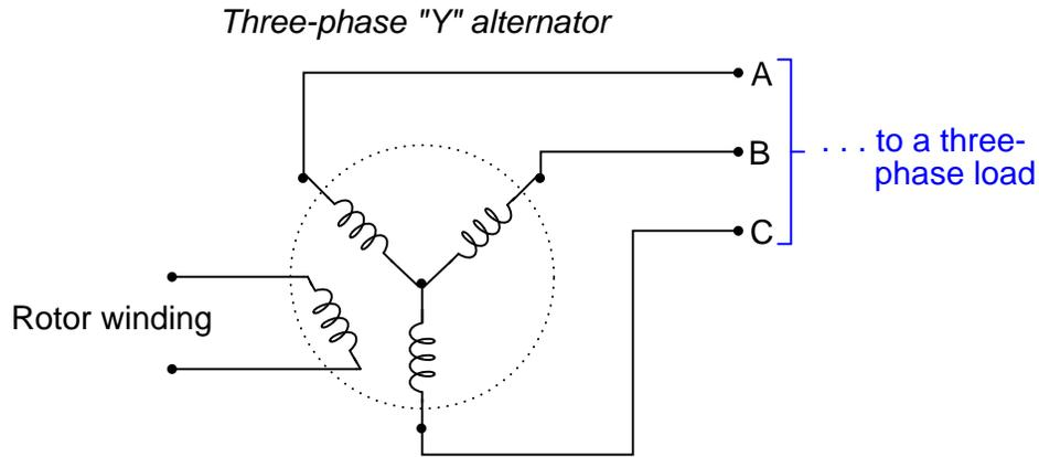
How much AC voltage will appear between any two of the lines ( $V_{AB}$ ,  $V_{BC}$ , or  $V_{AC}$ ) if each stator coil inside the alternator outputs 277 volts? Draw a phasor diagram showing how the phase (winding) and line voltages relate.
