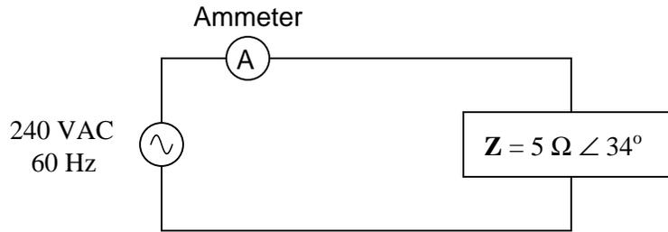
Now, calculate the line current and power factor for the same circuit after the addition of a capacitor in parallel with the load:
