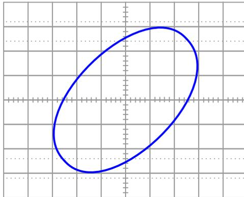
From this figure, calculate the phase angle ( $\Theta$ ) and the power factor for this motor circuit.
