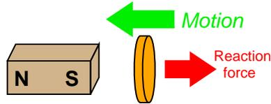
We know this force is magnetic in nature. That is, the induced current causes the disk itself to *become* a magnet in order to react against the permanent magnet's field and produce the opposing force. For each of the following scenarios, label the disk's induced magnetic poles (North and South) as it reacts to the motion imposed by an outside force:
