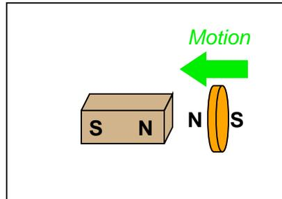
Follow-up question: trace the direction of rotation for the induced electric current in the disk necessary to produce both the repulsive and the attractive force.
