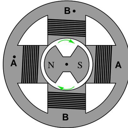
Each pair of windings in each set is series-connected, so they act as just two separate windings:
