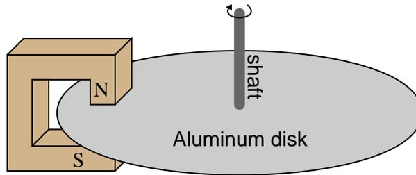
The disk itself need not be made of a ferromagnetic material in order for the magnet to create a "drag" force. It simply needs to be a good conductor of electricity.
