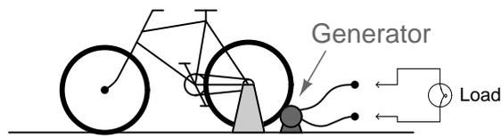
The person pedaling this bicycle/generator notices that it becomes more difficult to pedal when the generator is connected to a load such as a light bulb, or when it is charging a battery. When the generator is open-circuited, however, it is very easy to spin. Explain why this is, in terms of *work* and energy transfer.
