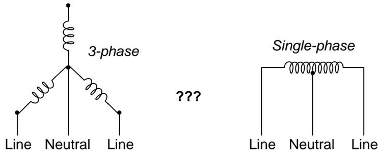
An experienced electrician suggests you build the following circuit to test whether or not the home's power is supplied by a 3-phase source or a single-phase source:
