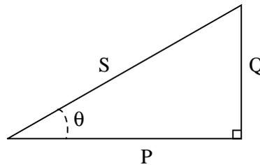
Explain what happens to the triangle if power factor correction components are added to a circuit. What side(s) change length on the triangle, and what happens to the angle  $\theta$ ?
