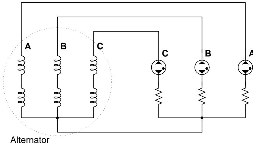
If the alternator spins fast enough (clockwise, as shown), the AC voltage induced in its windings will be enough to cause the neon lamps to "blink" (neon bulbs have very fast reaction times and thus cannot maintain a glow for very long without current, unlike incandescent lamps which operate on the principle of a glowing-hot metal filament). Most likely this blinking will be too fast to discern with the naked eye.
