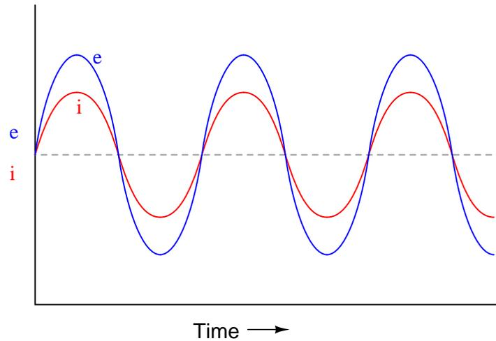
Given that power is the product of voltage and current ( $p = ie$ ), plot the waveform for power in this circuit.
