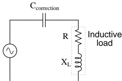
Explain why series capacitance is not considered a practical solution for power factor correction in most applications.
