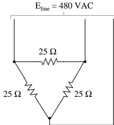
One more question: write an equation for calculating power in a balanced, three-phase circuit, given line voltage and line current only.
