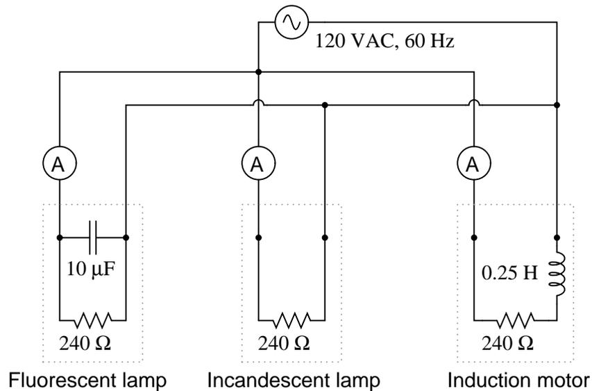
If someone were to read each of the ammeters' indications and multiply the respective currents by the figure of 120 volts, would the resulting power figures ( $P = IE$ ) agree with the actual power dissipations? Explain why or why not, for each load.
