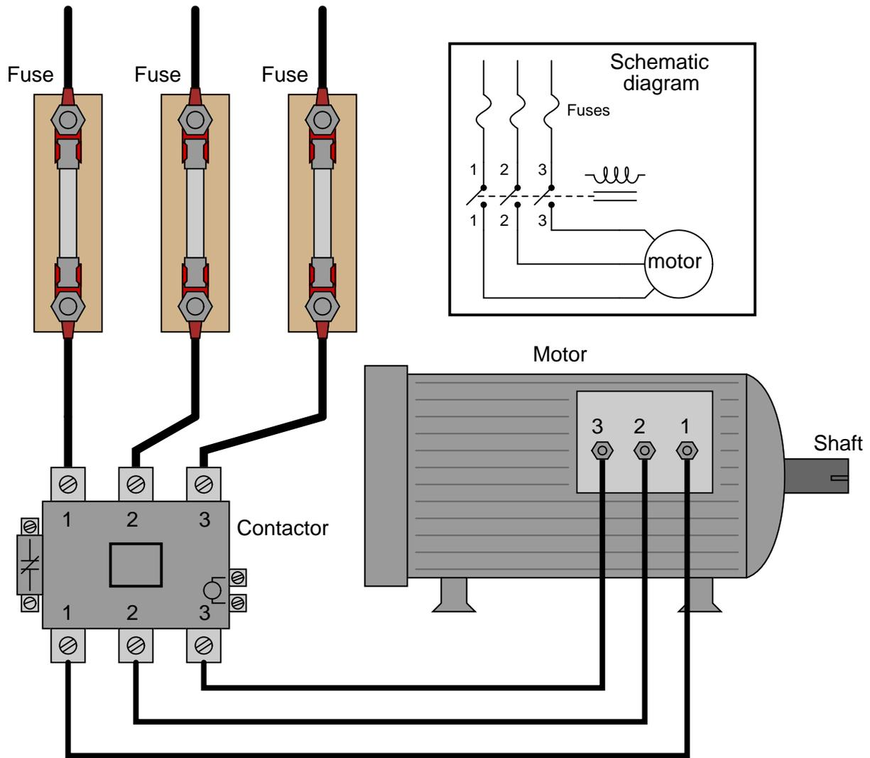
After years of faithful service, one day this motor refuses to start. It makes a "humming" sound when the contactor is energized (relay contacts close), but it does not turn. A mechanic checks it out and determines that the shaft is not seized, but is free to turn. The problem must be electrical in nature!
