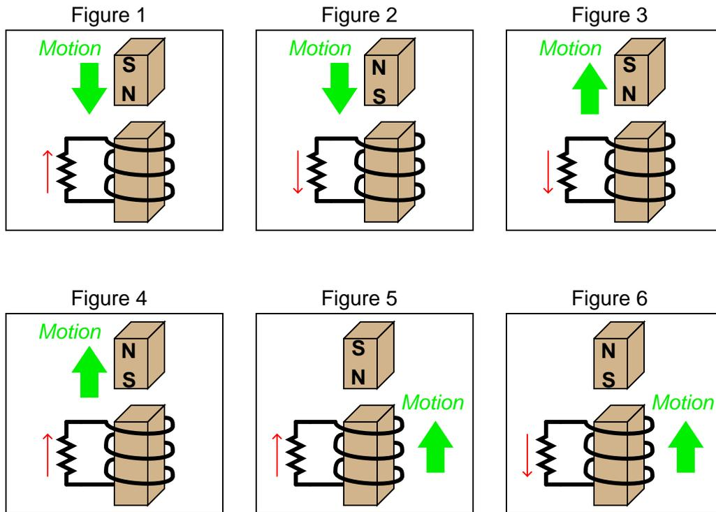
*Note: all current directions shown using conventional flow notation (following the right-hand rule)*
