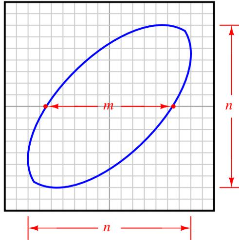
Determine what the formula is for calculating the phase shift angle for this circuit, given these dimensions. Hint: the formula is trigonometric! If you don't know where to begin, recall what the respective Lissajous figures look like for a  $0^\circ$  phase shift and for a  $90^\circ$  phase shift, and work from there.
