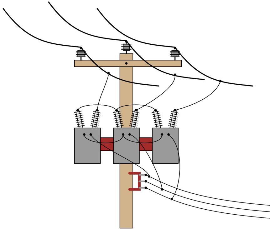
Of course, this is not the only way these three transformers could be connected in a Y-Y configuration.
