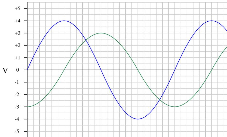
If the 4-volt (peak) sine wave is denoted in phasor notation as  $4 \text{ V} \angle 0^\circ$ , how should the 3-volt (peak) waveform be denoted? Express your answer in both polar and rectangular forms.
