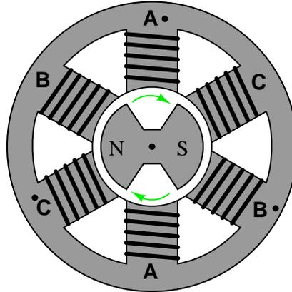
Each pair of windings in each set is series-connected, so they act as just three separate windings (pay close attention to the phase-marking dots!):
