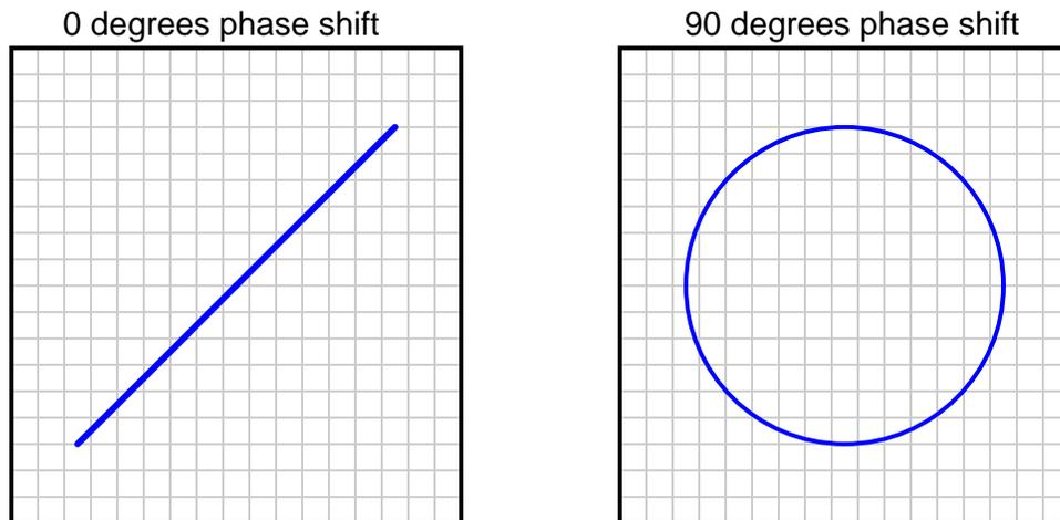
Challenge question: what kind of Lissajous figures would be plotted by the oscilloscope if the signals were non-sinusoidal? Perhaps the simplest example of this would be two square waves instead of two sine waves.
