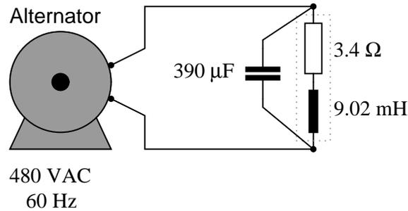
Follow-up question: when we use capacitors as power factor correction components in an AC power system, the equivalent series resistance (ESR) inside the capacitor becomes a significant factor:
