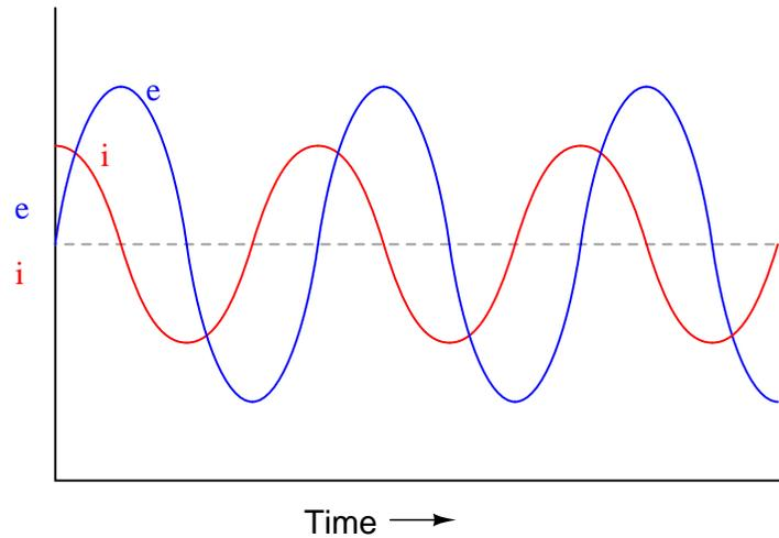
Given that power is the product of voltage and current ( $p = ie$ ), plot the waveform for power in this circuit. Also, explain how the mnemonic phrase "*ELI the ICE man*" applies to these waveforms.
