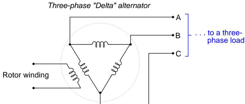
How much AC current will each of the lines ( $I_A$ ,  $I_B$ , or  $I_C$ ) conduct to a load (not shown) if each stator coil inside the alternator outputs 17 amps of current?
