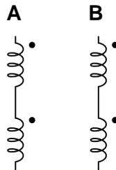
If one end of each winding pair were connected together at a common ground point, and each winding pair output 70 volts RMS, how much voltage would be measured between the open winding pair ends?
