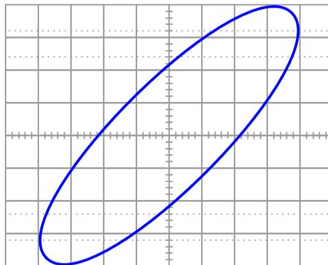
Calculate the power factor of the AC motor from this oscilloscope display.
