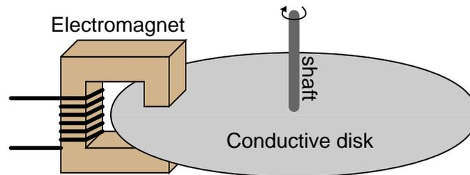
Follow-up question: describe some of the advantages and disadvantages that a magnetic brake would have, compared to mechanical brakes (where physical contact produces friction on the shaft).
