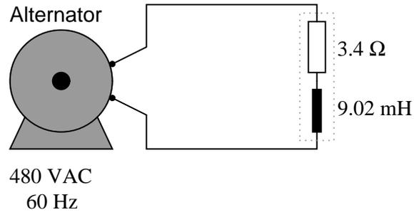
Then, calculate the size of the capacitor necessary to "correct" the power factor to a value of 1.0, showing the best location of the capacitor in the circuit.
