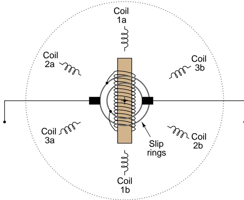
Explain how this motor can be operated as either a synchronous motor or a "plain" induction motor.
