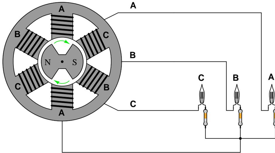
The schematic diagram for this alternator/lamp system is as follows:
