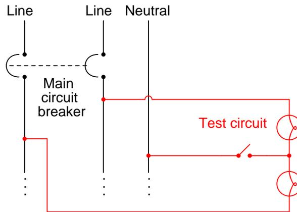
The electrician tells you to open and close the switch, and observe the brightness of the light bulbs. This will indicate whether or not the system is 3-phase.
