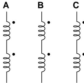
If one end of each winding pair were connected together at a common ground point, and each winding pair output 70 volts RMS, how much voltage would be measured between any two open wires?
