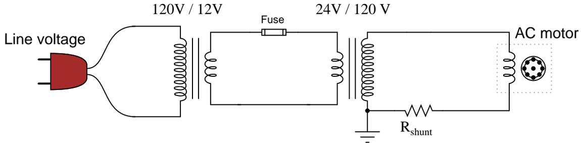
This circuit ensures the motor only receives about 60 volts, reducing shock hazard somewhat and allowing the use of capacitors rated for 100 volts (a common mylar capacitor rating). The smaller the motor, the less capacitance will be required to correct for power factor. Remind your students that the capacitors used in this exercise must be *non-polarized*, since they must operate on AC and not DC!
