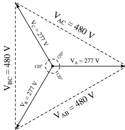
Follow-up question #1: what is the ratio between the line and phase voltage magnitudes in a Y-connected three-phase system?
