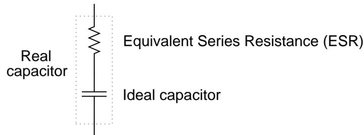
Current through this equivalent series resistance produces heat, and when we're dealing with MVARs worth of reactive power in high-current circuits, this heat can be substantial unless ESR is held low by special capacitor designs. Describe some possible hazards of excessive ESR for a power factor correction capacitor in a high-current circuit.
