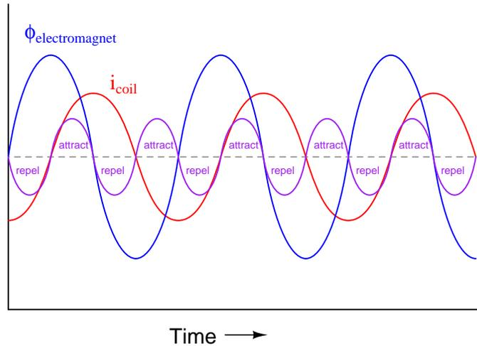
Note the equal-amplitude attraction and repulsion peaks shown on the graph.
