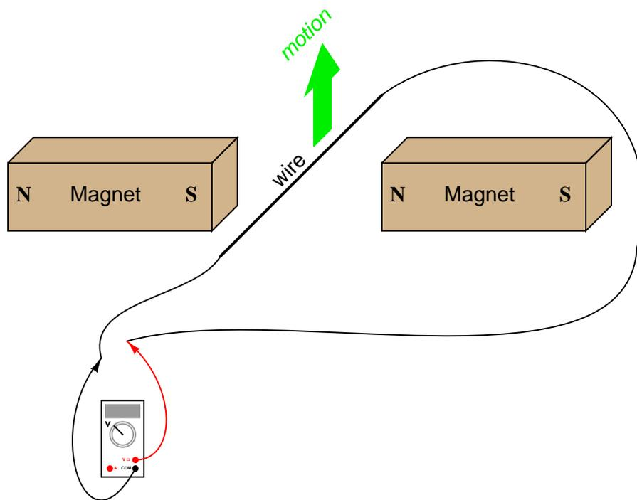
Describe the factors influencing the magnitude of the voltage induced by motion, and determine whether this is an example of an electric *motor* or an electric *generator*.
