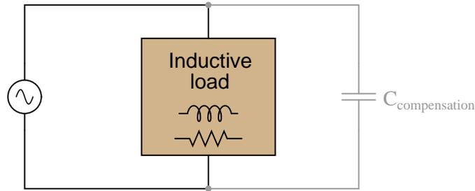
Define a step-by-step procedure for calculating the size of compensating capacitor needed (in Farads) in order to correct any lagging power factor to a value of unity. Make your procedure general enough that it may apply to any scenario.
