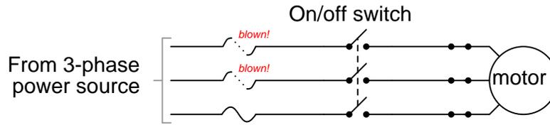
When the on/off switch was closed again, the motor made a loud "humming" noise, then became quiet after a few seconds. It never turned, though. Upon inspection, the electrician discovered the same two fuses had blown again.
