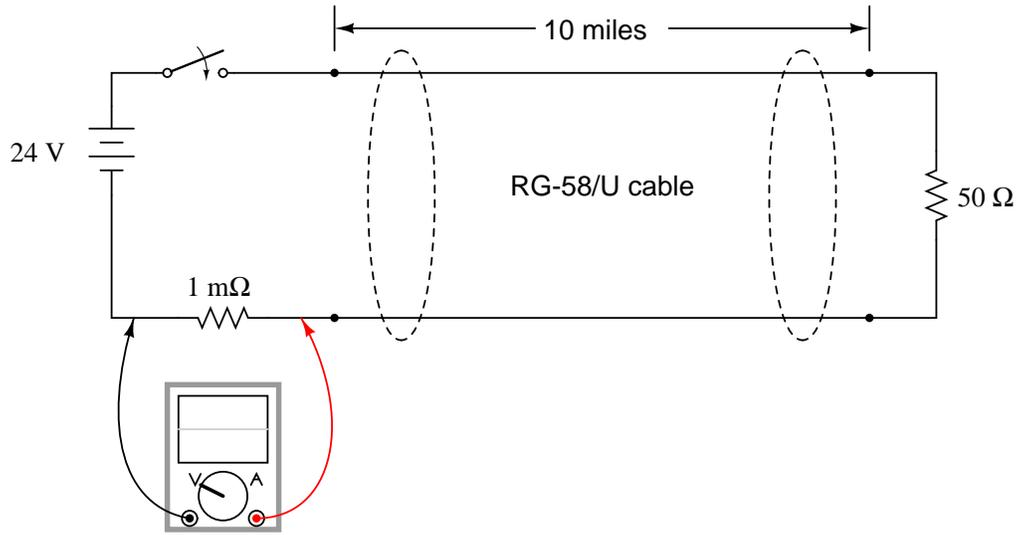
What sort of waveform or pulse would the oscilloscope register after switch closure?
