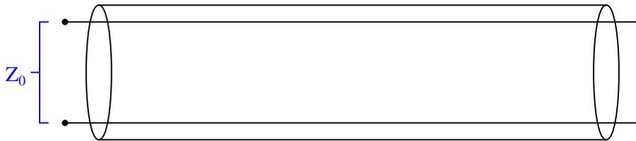
What would happen to the value of this characteristic impedance if we were to make the cable narrower, so that the conductors were closer together, all other dimensions remaining the same?
