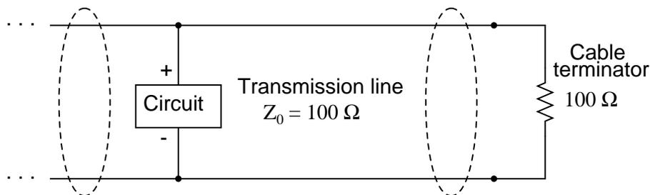
However, if we were to terminate the cable as shown, the termination resistor would dissipate a substantial amount of power. This is wasted energy, and would unnecessarily burden the power supply providing DC power to the network cable.
