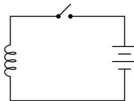
Like the resistor circuit, the coil will "seek" to achieve voltage equilibrium with the voltage source once the switch is closed. However, we know that the voltage induced in a coil is not directly proportional to current as it is with a resistor – instead, a coil's voltage drop is proportional to the *rate of change of magnetic flux over time* as described by Faraday's Law of electromagnetic induction:
