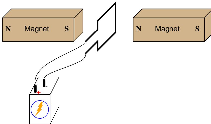
To increase the torque generated by the wire loop, you could use a loop with more than 1 "turn" of wire. This is not the only solution, though.
