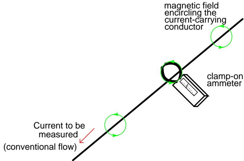
Knowing the principle behind this meter's operation, describe what current values will be indicated by the three clamp-on ammeters in this circuit:
