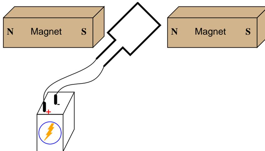
If this experiment is carried out, it may be found that the torque generated is quite small without resorting to high currents and/or strong magnetic fields. Devise a way to modify this apparatus so as to generate stronger torques using modest current levels and ordinary magnets.
