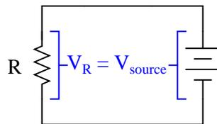
If the resistor is viewed as a source of voltage seeking equilibrium with the voltage source, then current *must* converge at whatever value necessary to generate the necessary balancing voltage across the resistor, according to Ohm's Law ( $V = IR$ ). In other words, *the resistor's current achieves whatever magnitude it has to in order to generate a voltage drop equal to the voltage of the source.*
