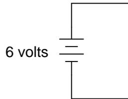
Suppose I short-circuited a 6-volt battery in the manner just described and found that the wire used to make the short-circuit gets warm after just a few seconds of carrying this current. Does this data agree or disagree with your predictions?
