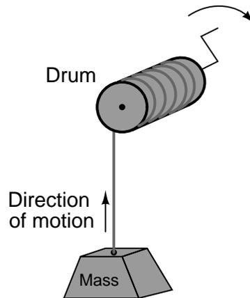
A physicist would likely look at this scenario as an example of energy exchange: the person turning the drum is expending energy, which in turn is being *stored* in the mass in potential form.
