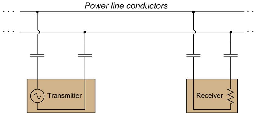
While coupling capacitors alone are adequate to perform the necessary filtering function needed by the communications equipment (to prevent damaged from the high-voltage electrical power also carried by the lines), that signal coupling may be made more efficient by the introduction of two *line tuning* units:
