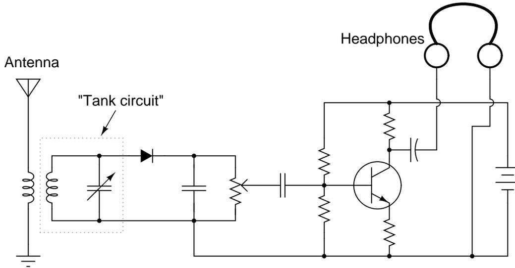
The "tank circuit" formed of a parallel-connected inductor and capacitor network performs a very important filtering function in this circuit. Describe what this filtering function is.
