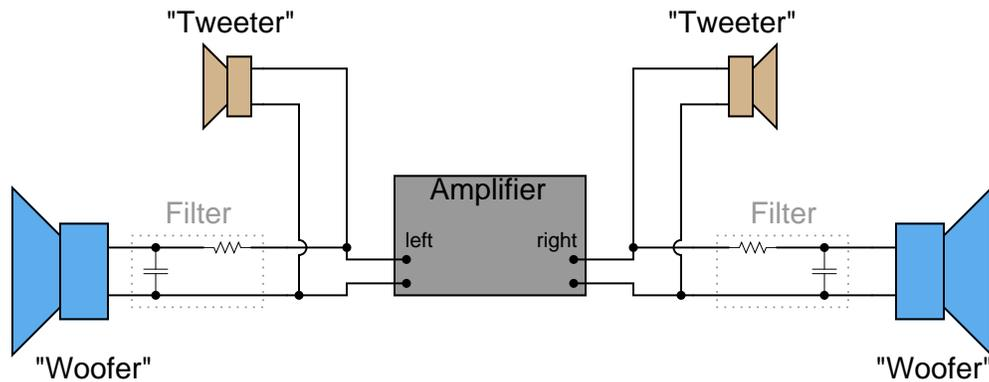
After examining this schematic, you see that your friend has the right idea in mind, but implemented it incorrectly. These filter circuits would indeed block high-frequency signals from getting to the woofers, but they would not actually accomplish the stated goal of minimizing wasted power.
