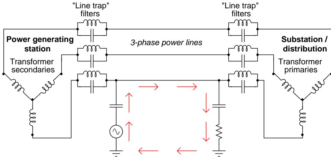
Follow-up question #1: trace the path of line-frequency (50 Hz or 60 Hz) load current in this system, identifying which component of the line trap filters ( $L$  or  $C$ ) is more important to the passage of power to the load. Remember that the line trap filters are tuned to resonate at the frequency of the communication signal (50-150 kHz is typical).
