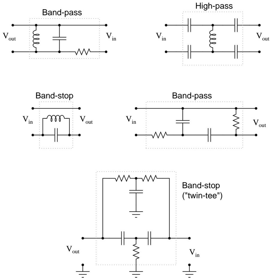
Unlike low-pass and high-pass filters, band-pass and band-stop filter circuits have *two* cutoff frequencies ( $f_{c1}$  and  $f_{c2}$ )!
