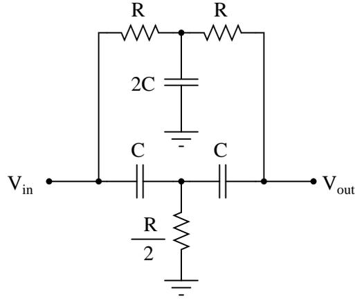
Research the equation predicting this circuit's "notch" frequency, given the component value ratios shown.
