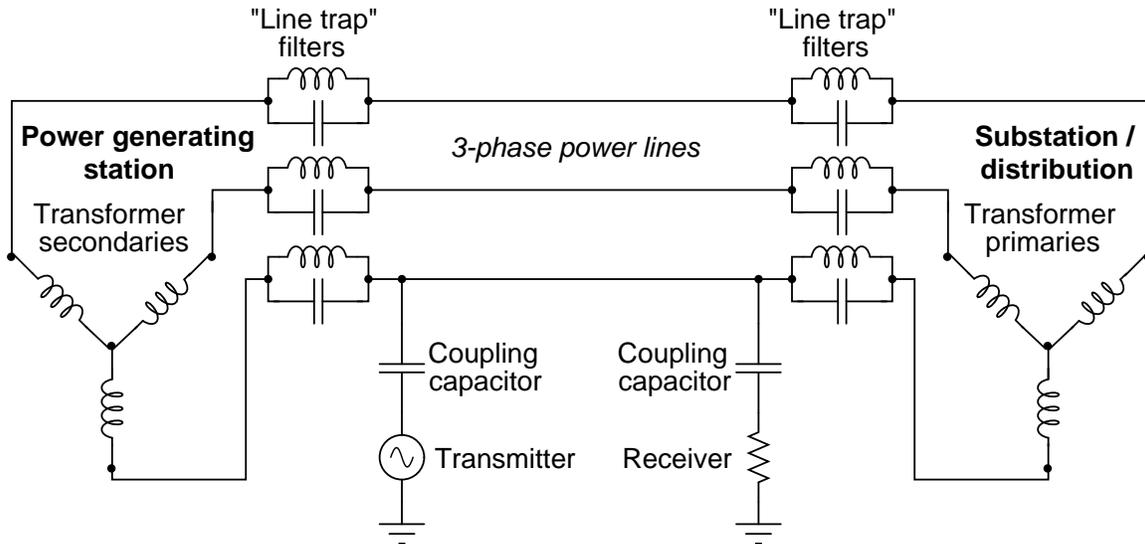
The communications transmitter is shown in simplified form as an AC voltage source, while the receiver is shown as a resistor. Though each of these components is much more complex than what is suggested by these symbols, the purpose here is to show the transmitter as a *source* of high-frequency AC, and the receiver as a *load* of high-frequency AC.
