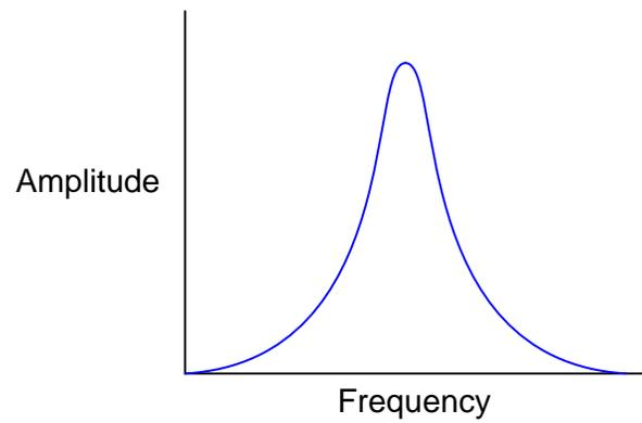
The bandwidth of a band-pass filter circuit is that range of frequencies where the output amplitude is at least 70.7% of maximum:
