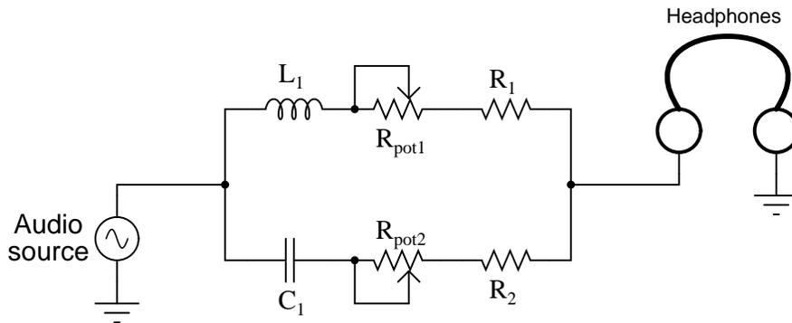
Suppose that after working just fine for quite a long while, suddenly no more bass tones were heard through the headphones. Identify at least two component or wiring faults that could cause this to happen.
