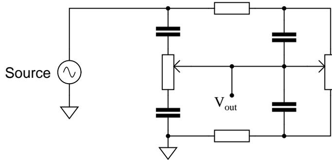
Determine which potentiometer controls the bass (low frequency) tones and which controls the treble (high frequency) tones, and explain how you made those determinations.
