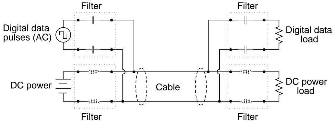
Follow-up question #1: how might the *superposition theorem* be applied to this circuit, for the purposes of analyzing its function?
