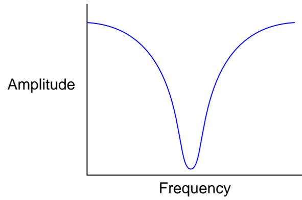
The bandwidth of a band-stop filter circuit is that range of frequencies where the output amplitude is reduced to at least 70.7% of full attenuation:
