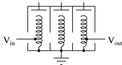
The above illustration shows a three-stage helical resonator, with adjustable metal plates at the top of each helix for tuning. Draw a schematic representation of this resonator, and explain where the capacitance comes from that allows each of the coils to form a resonant circuit.
