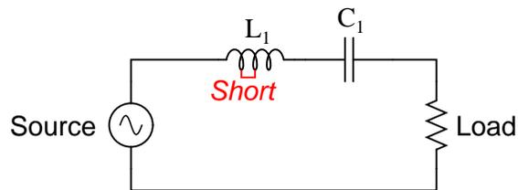
What sort of effect would this fault have on the filtering action of this circuit?
