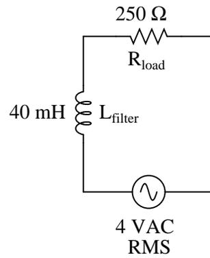
What do these figures tell you about the nature of this filter circuit (whether it is a low-pass or a high-pass filter), and also about the definition of *cutoff frequency* (also referred to as  $f_{-3dB}$ )?
