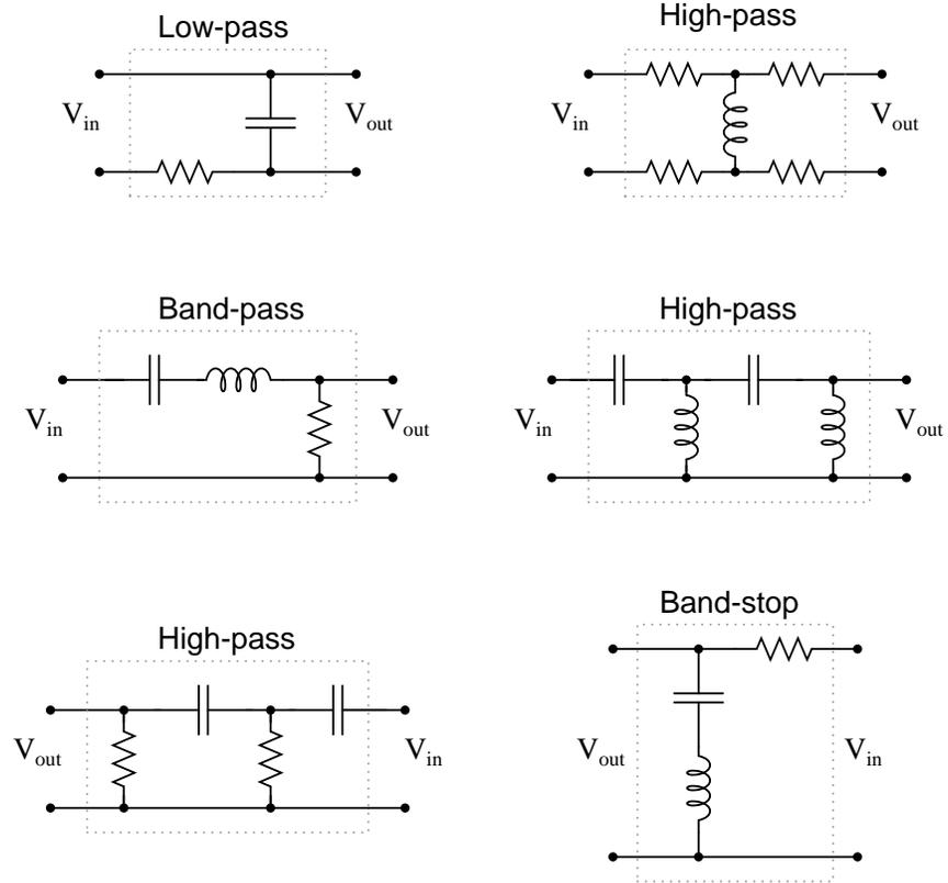
Follow-up question: in each of the circuits shown, identify at least one *single* component failure that has the ability to prevent any signal voltage from reaching the output terminals.
