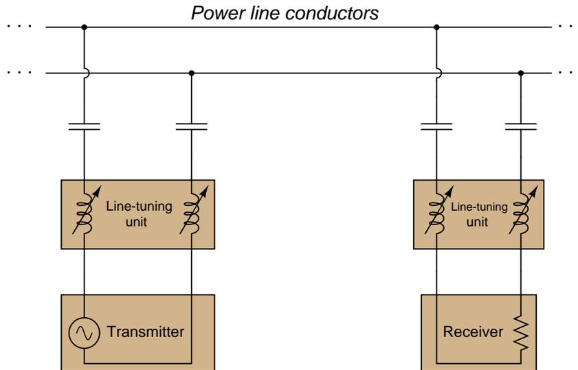
Explain why the addition of more components (in series, no less!) provides a better "connection" between the high-frequency Transmitter and Receiver units than coupling capacitors alone. Hint: the operating frequency of the communications equipment is fixed, or at least variable only over a narrow range.
