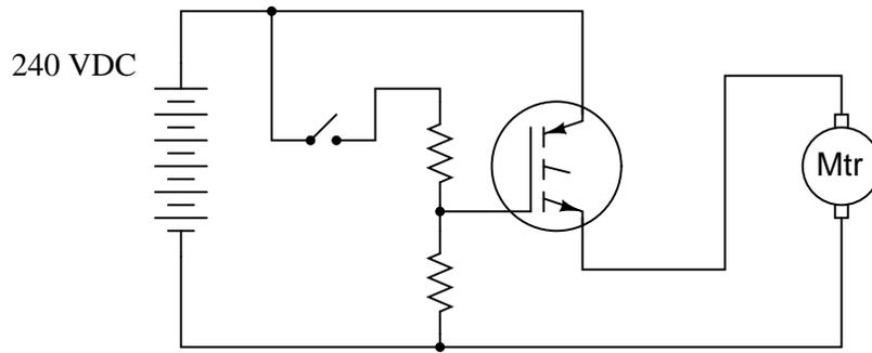
Follow-up question: calculate the values necessary for the two resistors shown, to provide a gate-to-emitter voltage of 10 volts, using 1/2 watt resistors.
