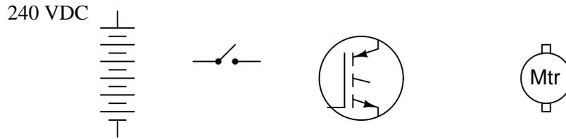
Note: the DC power supply voltage is 240 VDC, and the IGBT's maximum gate-to-emitter control voltage is 20 volts!
