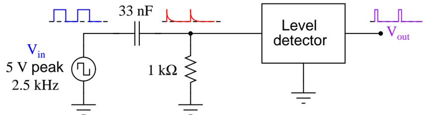
Each time the differentiator's output voltage signal spikes up to +5 volts and quickly decays to 0 volts, it causes the level detector circuit to output a narrow voltage pulse, which is what we want.
