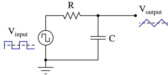
Anyone familiar with RC circuits will realize, however, that a passive integrator will not output a true triangle wave, but rather it will output a waveshape with "rounded" leading and trailing edges:
