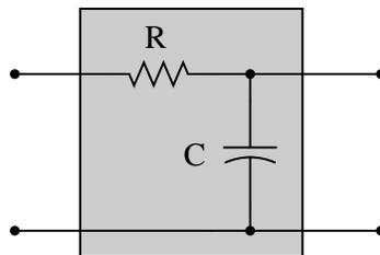
What specific type of passive filter does a passive integrator circuit resemble? Is the resemblance the same for LR integrators as well, or just RC integrators? What does this resemblance tell you about the frequency response of a passive integrator circuit?
