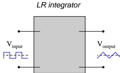
In addition to completing the inductor circuit schematic, qualitatively state the preferred values of  $L$  and  $R$  to achieve an output waveform most resembling a true triangle wave. In other words, are we looking for a large or small inductor; a large or small resistor?
