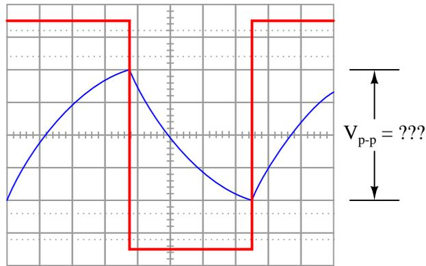
Hint: the output waveform will be centered exactly half-way between the two peaks of the input square wave as shown in the oscilloscope image. Do *not* base your answer on relative sizes of the two waveforms, as I have purposely skewed the calibration of the oscilloscope screen image so the two waveforms are not to scale with each other.
