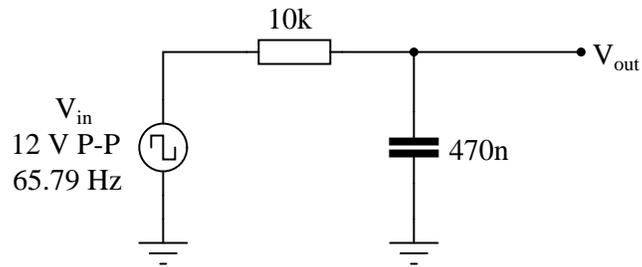
Determine the peak-to-peak voltage of the output waveform:
