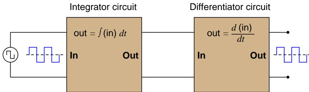
Based on what you know about differentiation and differentiator circuits, what must the signal look like in between the integrator and differentiator circuits to produce a final square-wave output? In other words, if we were to connect an oscilloscope in between these two circuits, what sort of signal would it show us?
