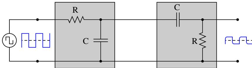
You recognize one of the RC networks as a passive integrator, and the other as a passive differentiator. What does the likeness of the output waveform compared to the input waveform indicate to you about differentiation and integration as *functions* applied to waveforms?
