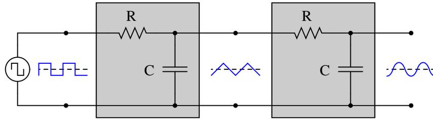
From Fourier's theory, we know that a square wave is nothing more than a series of sinusoidal waveforms: the fundamental frequency plus all odd harmonics at diminishing amplitudes. Looking at the two integrators as *passive filter circuits*, explain how it is possible to get a pseudo-sine wave from a square wave input as shown in the above diagram. Also, explain why the final output is not a true sine wave, but only resembles a sine wave.
