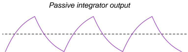
What can be done with the values of  $R$  and  $C$  to best approximate a true triangle wave? What variable must be compromised to achieve the most linear edges on the integrator output waveform? Explain why this is so.
