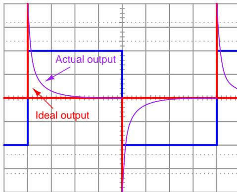
Follow-up question: given that  $R_{shunt} \ll X_C$  in order that the resistance does not impede the capacitor current to any significant extent, what does this suggest about the necessary time-constant ( $\tau$ ) of a passive differentiator circuit? In other words, what values of  $R$  and  $C$  would work best in such a circuit to produce an output waveform that is as close to ideal as possible?
