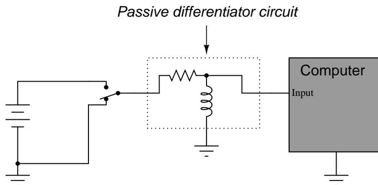
This circuit would certainly work to create brief pulses of voltage to the computer input, but it would also likely *destroy* the computer's input circuitry after a few switch actuations! Explain why.
