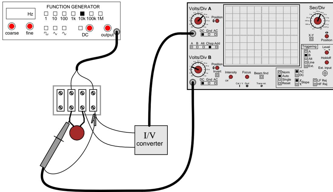
For each of the following voltage waveforms (channel B), plot the corresponding capacitor current waveform (channel A) as it would appear on the oscilloscope screen:
