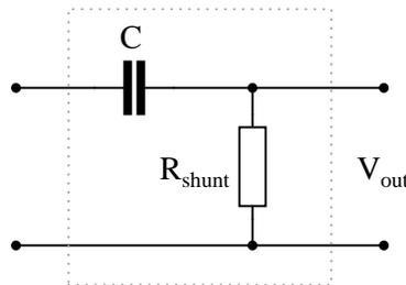
The resistor is called a *shunt* because it is designed to produce a voltage proportional to current, for the purpose of a parallel ("shunt")-connected voltmeter or oscilloscope to measure that current. Ideally, the shunt resistor is there only to help us measure current, and not to impede current through the capacitor. In other words, its value in ohms should be very small compared to the reactance of the capacitor ( $R_{shunt} \ll X_C$ ).
