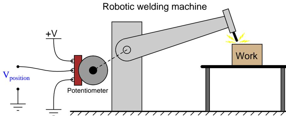
As the robotic arm rotates up and down, the potentiometer wire moves along the resistive strip inside, producing a voltage directly proportional to the arm's position. A voltmeter connected between the potentiometer wiper and ground will then indicate arm position. A computer with an analog input port connected to the same points will be able to measure, record, and (if also connected to the arm's motor drive circuits) control the arm's position.
