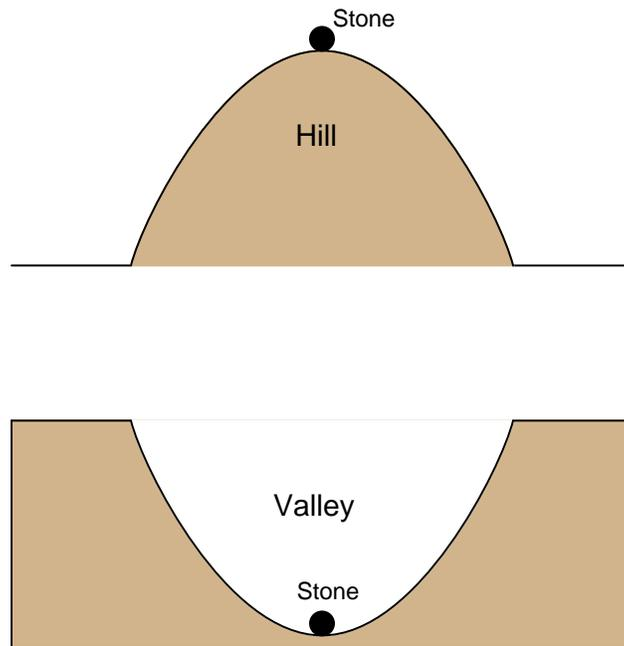
The stability of the stone in each of these scenarios represents the stability of a specific type of electrical feedback system. Which of these scenarios represents negative feedback, which represents positive feedback, and why?
