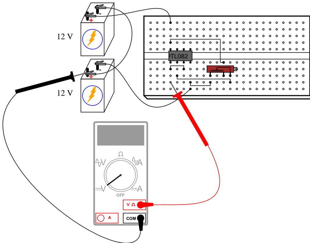
Draw a schematic diagram of this faulty circuit, and determine what the voltmeter's indication will be, explaining why it is such.
