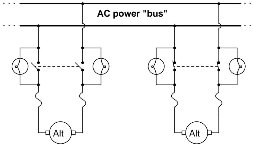
What should the alternator operator look for before closing the alternator switch? Do bright lights indicate a condition of being "in-phase" with the bus, or do dim lights indicate this? What does the operator have to do in order to bring an alternator into "phase" with the bus voltage?
