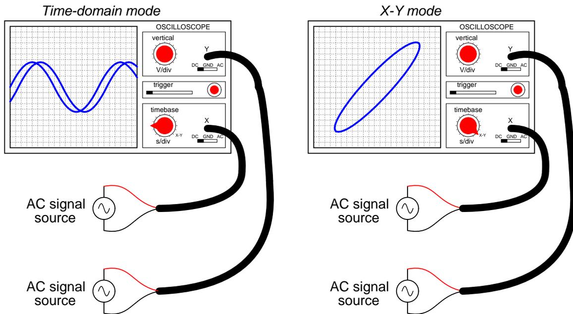
The oval pattern shown in the right-hand oscilloscope display of the above illustration is typical for two sinusoidal waveforms of the same frequency, but slightly out of phase with one another. The technical name for this type of  $X - Y$  plot is a *Lissajous figure*.
