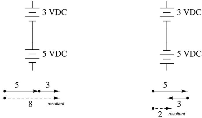
In the right-hand circuit, where the two voltage sources are opposing, one of the phasors will have an angle of  $0^\circ$ , while the other will have an angle of  $180^\circ$ .
