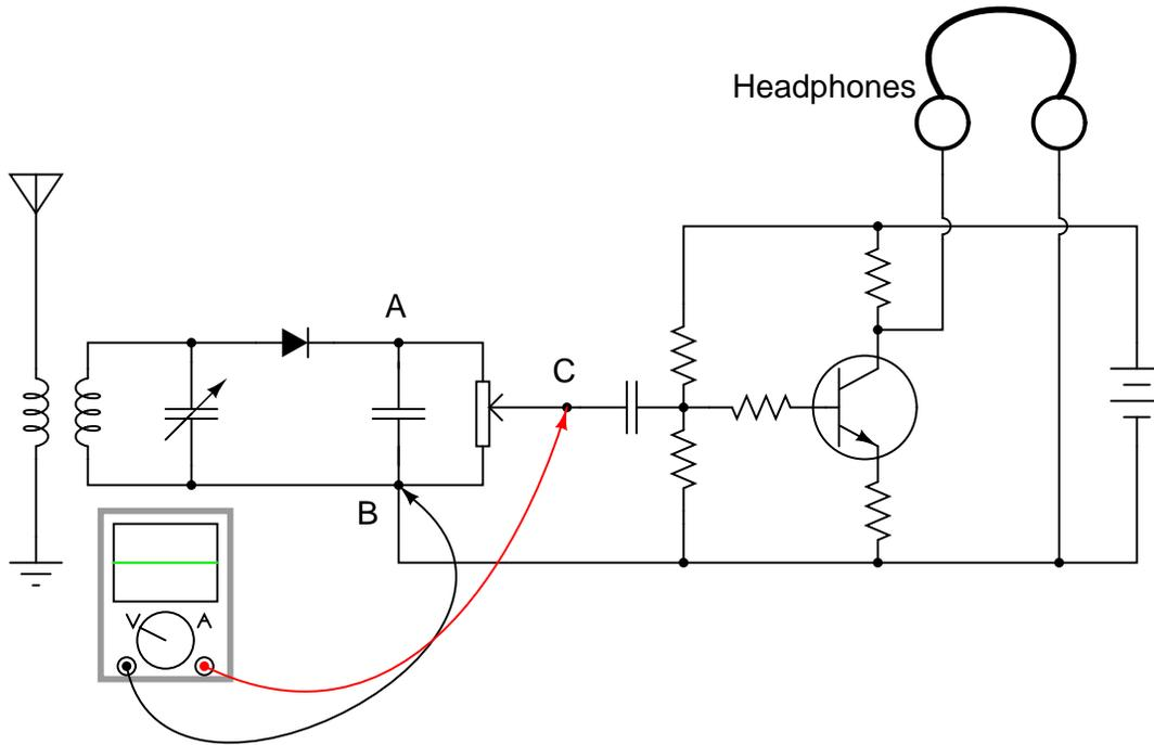
What do these voltage measurements indicate about the nature of the problem in the receiver circuit? Is there a general troubleshooting rule that may be drawn from this example? If so, what is it? If possible, identify the precise nature of the failure.
