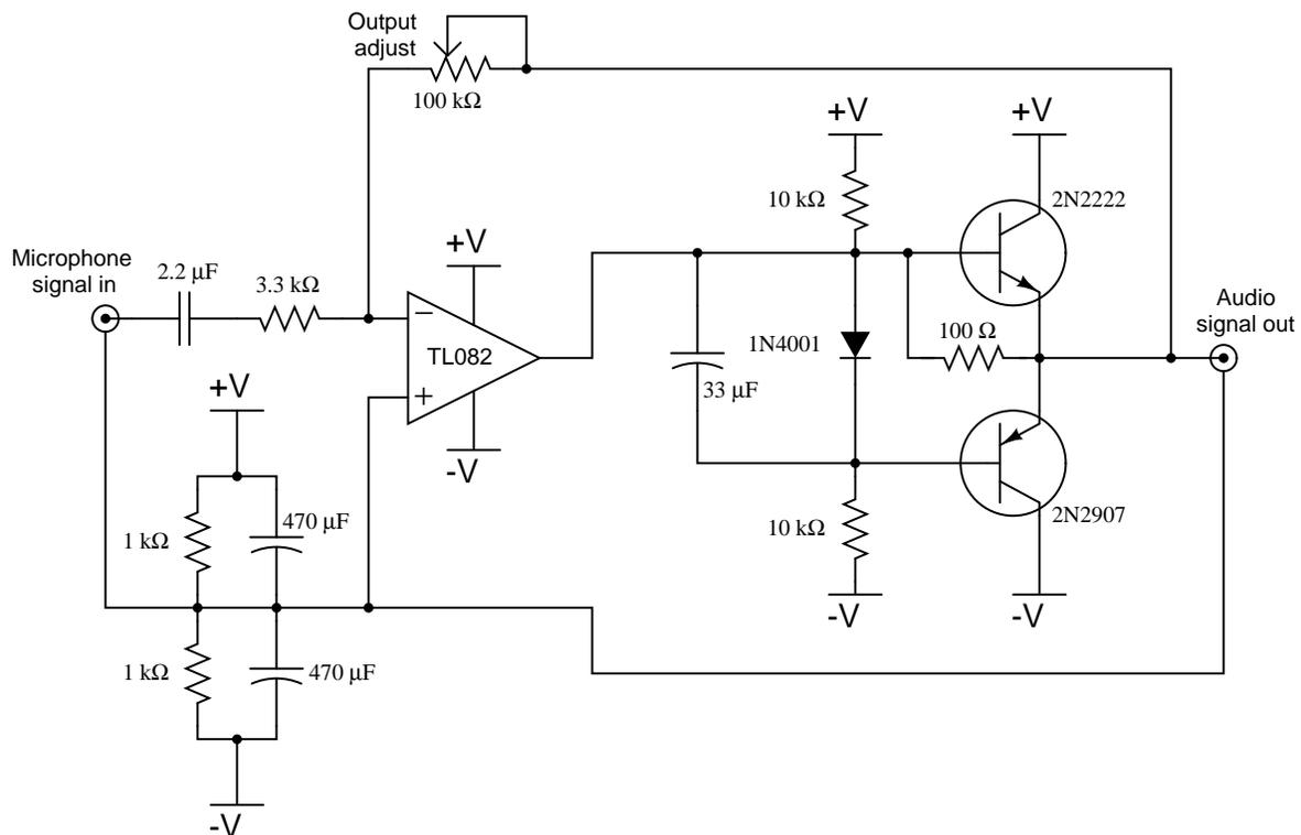
I have used power supply voltages of 12 volts (+V = +6 volts ; -V = -6 volts) and 24 volts (+V = +12 volts; -V = -12 volts), both with good success. Of course, you are not restricted to using this exact design – feel free to modify it!
