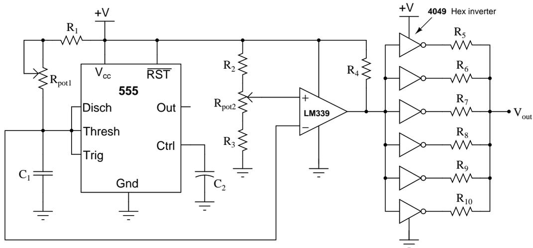
Here, six CMOS inverters (IC part number 4049) are ganged together in parallel to supply significantly more sourcing and sinking current capability than the LM339-with-pullup-resistor could on its own. Since CMOS logic gates are inherently on-or-off devices, they have no trouble handling the square wave output of the LM339.
