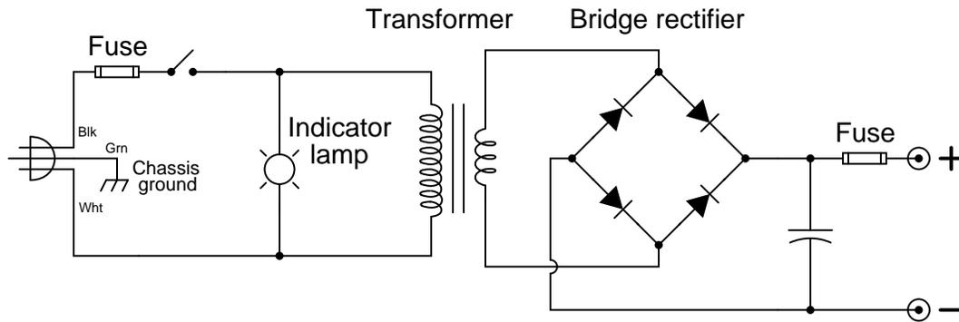
Of course, you are not restricted to using this exact design. One design feature I insist on, though, is that you build your own rectifier circuit from individual diodes, rather than use a packaged rectifier assembly. I highly recommend the use of "barrier strips" or "terminal strips" to make the electrical connections between components. These connection devices provide solid, permanent electrical connections while still allowing components to be easily installed and removed.
