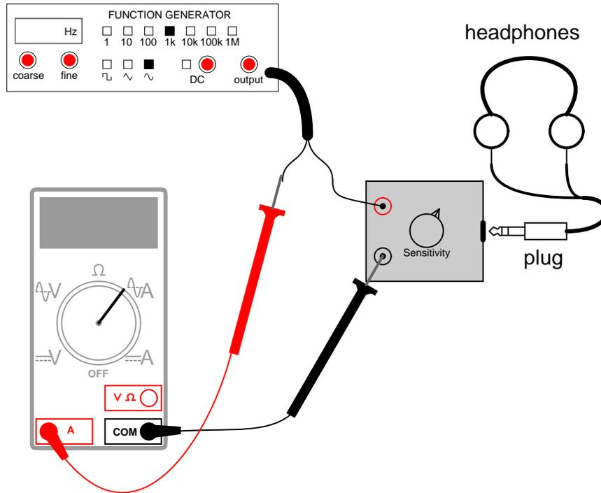
Compare this against the lowest amount of audible signal current for the headphones directly. Which component of the detector circuit is responsible for this increased sensitivity?
