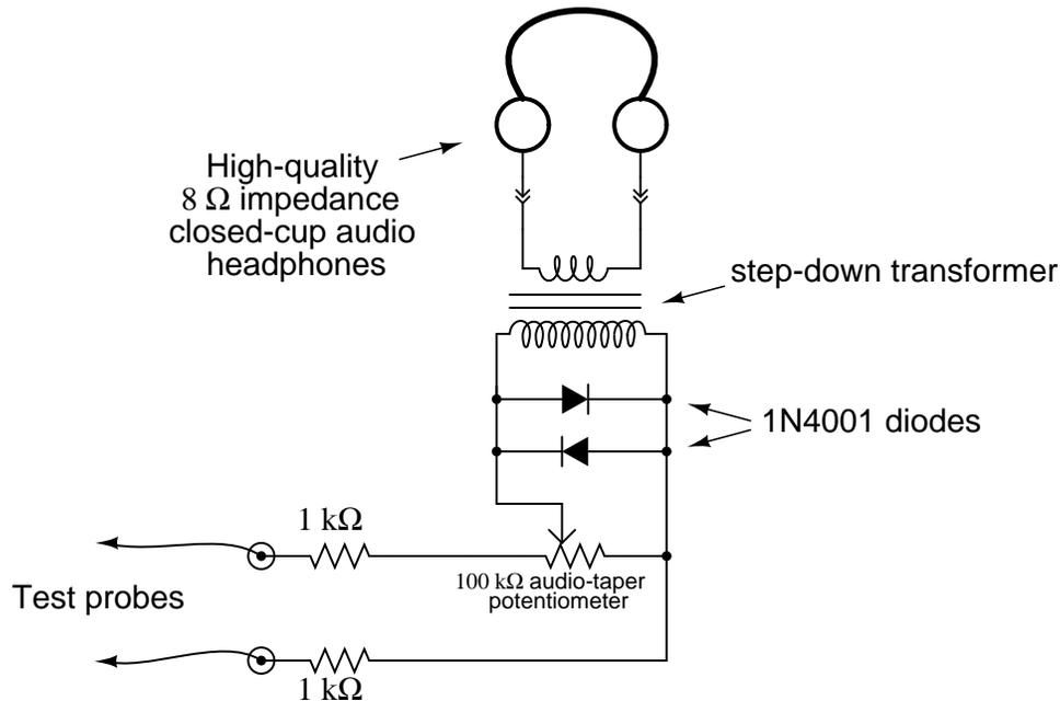
I recommend you follow this design closely, to ensure your detector will function in a safe manner. The headphones should be of the "passive" type, meaning no built-in amplifier or sound controls – just a plain set of 8 Ω closed-cup headphones. If you wish to make any design changes, please consult your instructor.
