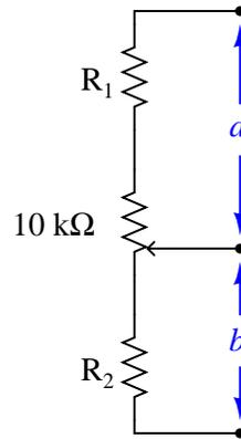
First, write an equation for each circuit, showing how resistances  $R_1$ ,  $R_2$ , and the  $10 \text{ k}\Omega$  of the potentiometer combine to form the ratio  $\frac{a}{b}$ . Then, use techniques for solving simultaneous equations to calculate actual resistance values for  $R_1$  and  $R_2$ .
