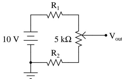
$V_{out} \text{ (minimum)} = 3 \text{ volts}$
