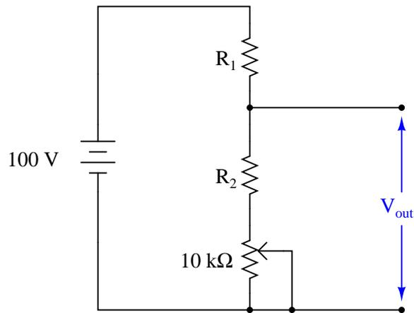
Desired range for  $V_{out} = 30 \text{ volts to } 70 \text{ volts}$
