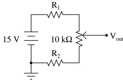
$$V_{out} \text{ (minimum)} = 5 \text{ volts} \quad V_{out} \text{ (maximum)} = 12 \text{ volts}$$
