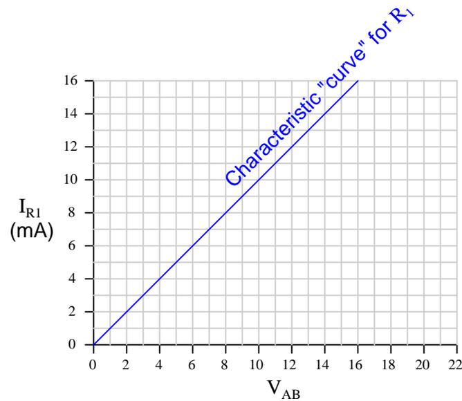
Next, I will plot the load line as defined by the 1.5 kΩ load resistor. This "load line" expresses the voltage available between the same two terminals ( $V_{AB}$ ) as a function of the load current, to account for voltage dropped across the load:
