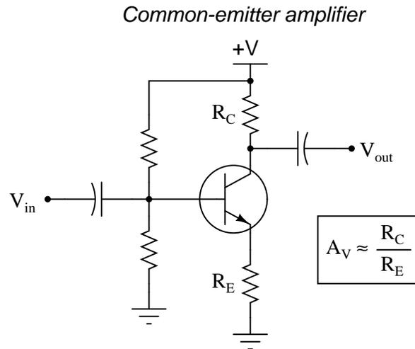
Knowing this, calculate the necessary resistance values for the following fixed-value resistors ( $R_1$  and  $R_2$ ) to give this common-emitter amplifier an adjustable voltage gain range of 4 to 7:
