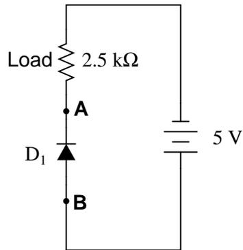
The diode's characteristic curve is already plotted on the following graph. Your task is to plot the load line for the circuit on the same graph, and note where the two lines intersect:
