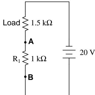
We will have to plot a load line for this simple two-resistor circuit along with the "characteristic curve" for resistor  $R_1$  in order to see the benefit of a load line. Load lines really only have meaning when superimposed with other plots. First, the characteristic curve for  $R_1$ , defined as the voltage/current relationship between terminals **A** and **B**:
