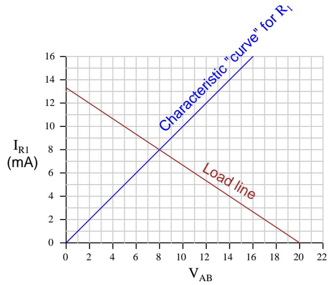
At what value of current ( $I_{R1}$ ) do the two lines intersect? Explain what is significant about this value of current.
