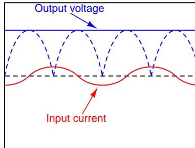
As you can see, the input current waveform lags the voltage waveform by  $90^\circ$ , because when the power supply is unloaded, the only input current is the *magnetizing current* of the transformer's primary winding.
