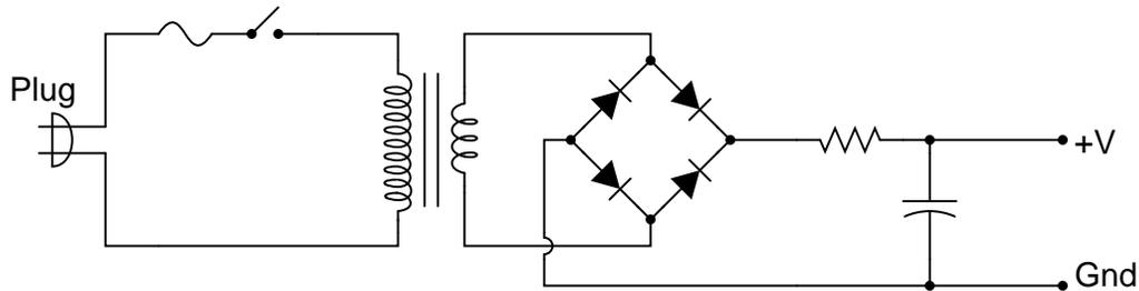
While this design will work, there are better filter configurations for this application. Describe the limitations of the circuit shown, and explain how some of the other filters would do a better job.
