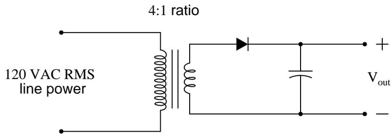
This comes as a surprise because the diode has a repetitive peak reverse voltage rating of 50 volts, which the technician knows is greater than the peak voltage output by the step-down transformer. However, the technician has overlooked something very important in this circuit design. Explain what the problem is, and how to solve it.
