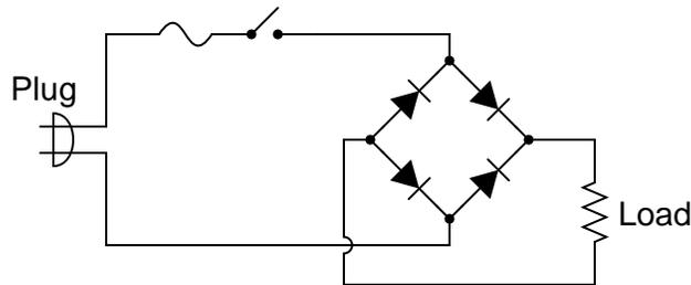
However, this form of AC-to-DC power conversion has some significant limits. Explain why most power supply circuits utilize a transformer instead of directly rectifying the line power as this circuit does.
