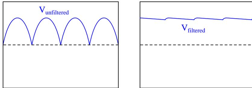
A low pass filter is the kind needed to filter "ripple voltage" from the power supply output.
