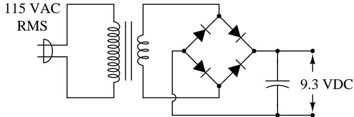
Explain why this is. How can the addition of nothing but a capacitor have such a great effect on the amount of DC voltage output by the circuit?
