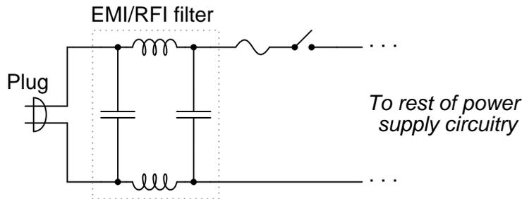
Determine what type of filter circuit this is (LP, HP, BP, or BS), and also determine the inductive and capacitive reactances of its components at 60 Hz, if the inductors are  $100 \mu\text{H}$  each and the capacitors are  $0.022 \mu\text{F}$  each.
