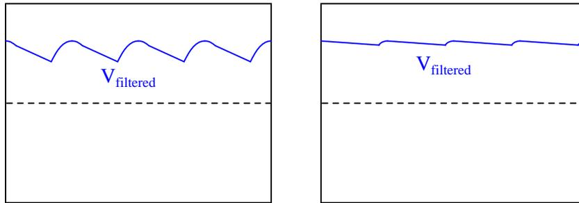
If both of these waveforms were measured on the same power supply circuit, at different times, determine which waveform was measured during a period of heavier "loading" (a "heavier" load being defined as a load drawing *greater* current).
