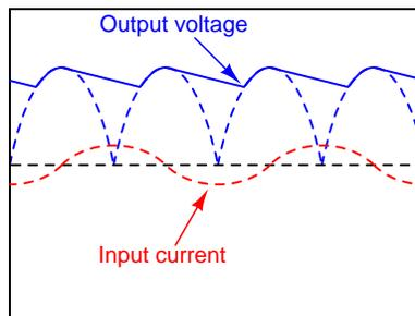
The non-filtered DC output waveform is still shown as a dotted line, for reference purposes.
