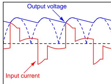
Challenge question: does the input current waveform shown here contain even-numbered harmonics (i.e. 120 Hz, 240 Hz, 360 Hz)?
