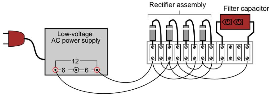
Incidentally, the "low voltage AC power supply" is nothing more than a step-down transformer with a center-tapped secondary winding.
