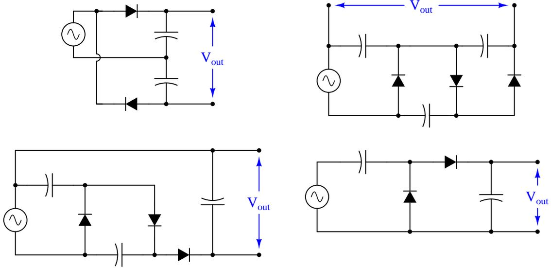
Determine the degree of voltage multiplication (double, triple, etc.) provided by each circuit.
