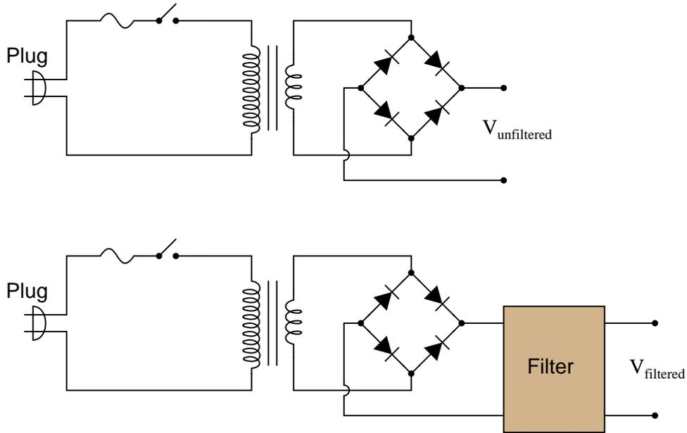
Draw the respective output voltage waveforms of these two power supply circuits ( $V_{unfiltered}$  versus  $V_{filtered}$ ). Also identify the type of filter circuit needed for the task (low pass, high pass, band pass, or band stop), and explain why that type of filter circuit is needed.
